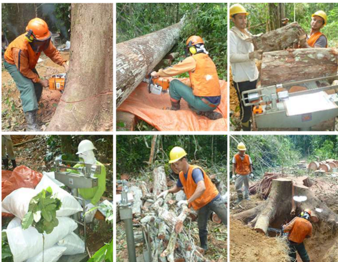
Figure 1. Images of Field Activities Using the Destructive Method for Determining Total Weight Above and Below the Soil of a Tree.
